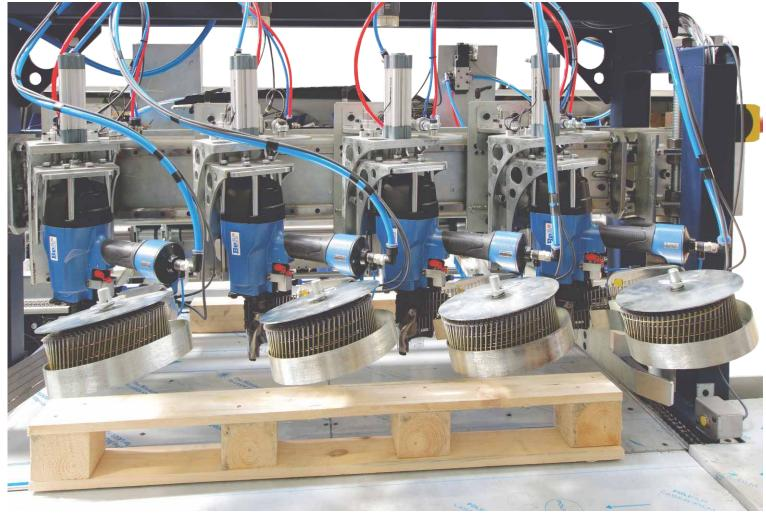
LEGPAL 1200 – automatic line for assembly of wooden shipping brackets
