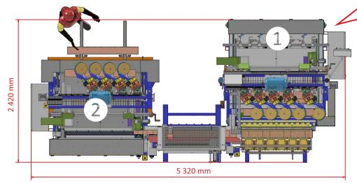
The first nailing unit (fixing blocks to the board)
