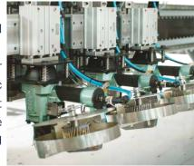
Two sets of molds can be placed on the worktable which allows the machine to work in cycles – when one set of molds is being fastened, one can perform the collection and loading of the other set. You can also program one nailing cycle over the entire length of the table with identical or different product molds.
